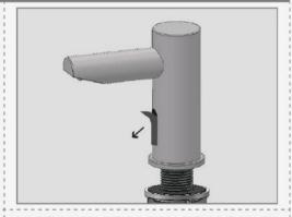
Connect the motor connector to its matching connector coming from the electronic unit. Please note that since the connector is water proof, some friction might apply.
